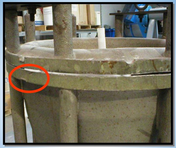
PL-S<sup>®</sup> forms a complete seal at the parting line. This prevents escape or entrance of internal and external gases.
