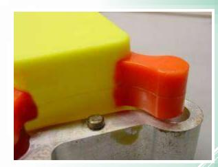
Hollow part now features solid, moulded in flanges for drilling and wall mounting.
